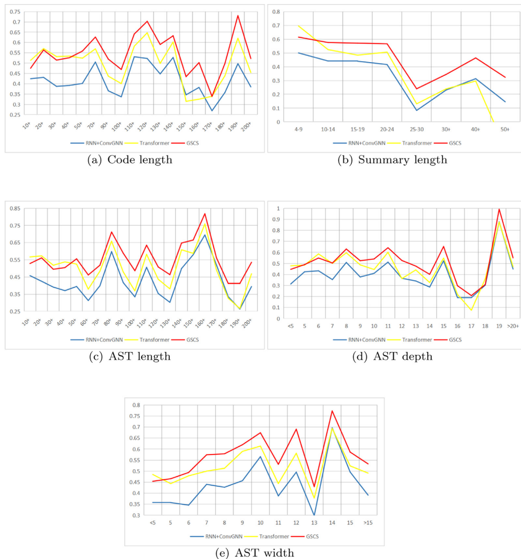
Fig. 5. The average BLEU-4 scores (standardized with a range from 0.3 to 0.6) for RNN+ConvGNN, Transformer, and GSCS as a function of code (a), and summary length (b) as well as AST length (c), depth (d), and width (e). We observe that the performance gap narrows as these metrics increase, however, we also observe GSCS consistently performing well at high values.
