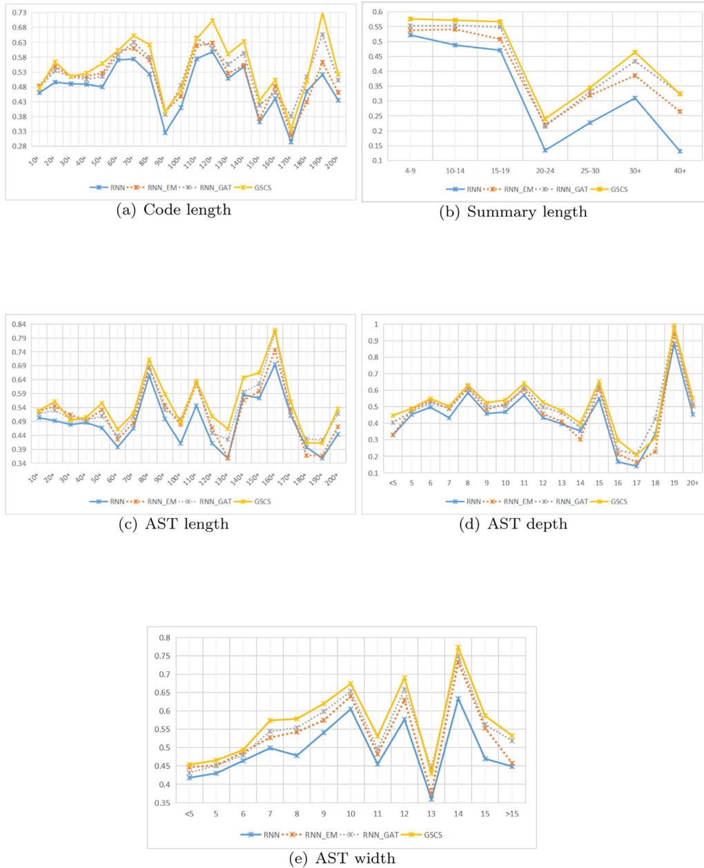
Fig. 6. The average BLEU-4 scores (standardized with a range from 0.3 to 0.6) for RNN, RNN_EM, RNN_GAT, and GSCS as a function of code (a), and summary length (b) as well as AST length (c), depth (d), and width (e).
