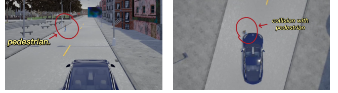
(a) Manipulating the ADS via the billboard to hit the pedestrian. (b) Collision occurred after the closed-loop manipulation.
